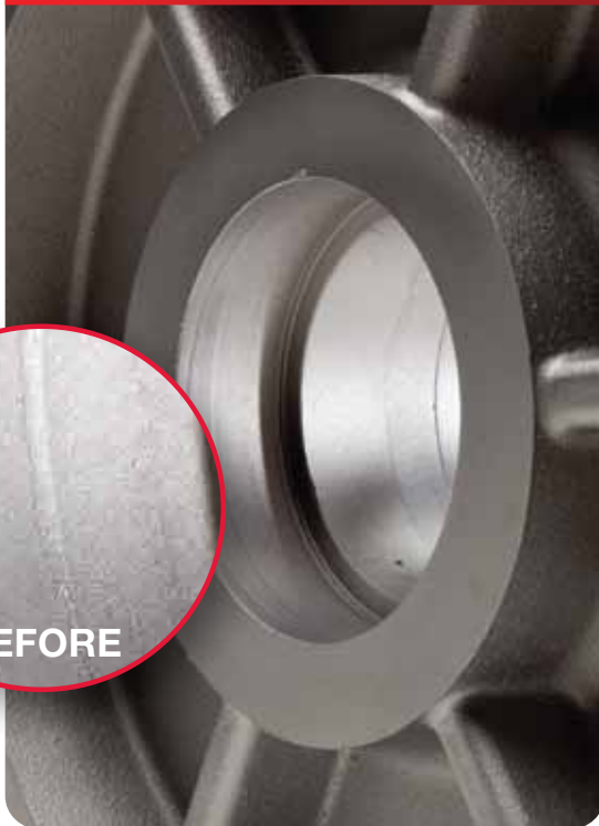
Oversized/damaged bearing bore from a spun bearing
