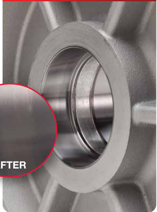
New steel insert in an aluminum hub
